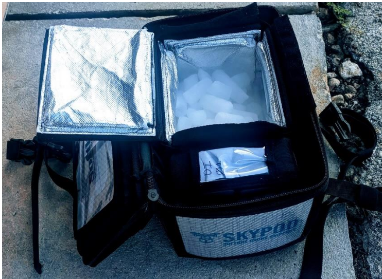
Figure 1: Softbox Systems Skypod with dry ice for -60C to -80C
