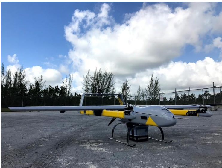
Figure 2: Volans-i VOLY C-10 vertical takeoff & landing aircraft
